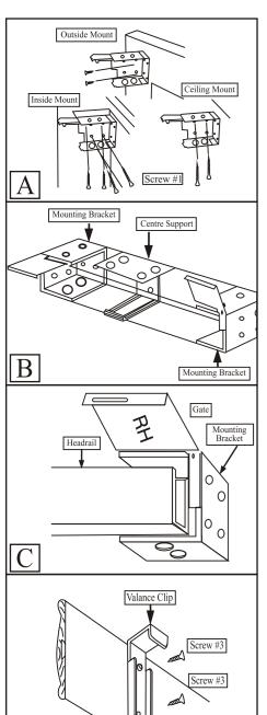
Brackets should be placed at the width of blind's head rail 6mm past each end. The bracket doesn't necessarily need to touch the inside face of the window frame.
