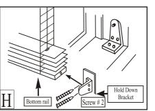
Hold down brackets: Using two small screws, screw hold down bracket to window facing or wall. Snap bracket pin ends into the hole at bottom rail end.
